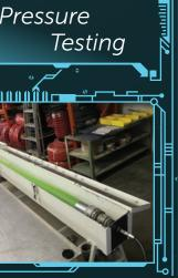
The final step of hose assembly is t confirm) that the hose is properly ested for its intended use. First, the hose is hooked into the test bench Once the bench is ready, the pressur nside the hose is increased to 150% o the optimal max working pressure o the hose. This pressure is then held fo a minimum of 5 minutes
