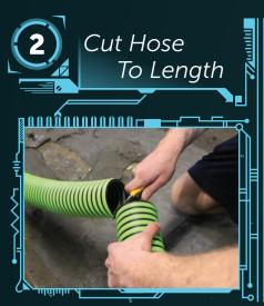
Once the hose is approved for us he hose is measured, then cut to the pecific length required for the hose The hose ends are cut smooth for an optimal connection to the fitting/and an anti-static wire is embedded i the hose, a small part of each wire is pulled free from the hose material and bent\_inwards. to\_ensure\_optimal connection to the fitting.
