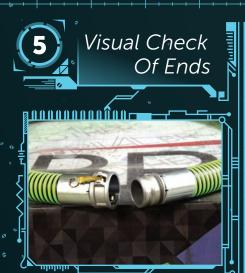
both ends are crimped, th ose assembly technician shecks each end for a proper crime This involves confirming that the interlock is correctly aligned, and that he width of the crimped hose conforms correctly pecification
