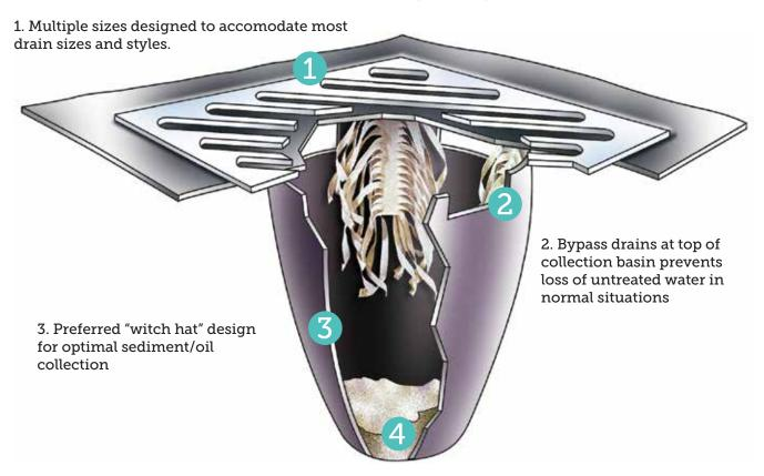
4. Filtering material allows water through but collects 80% + of contaminants
